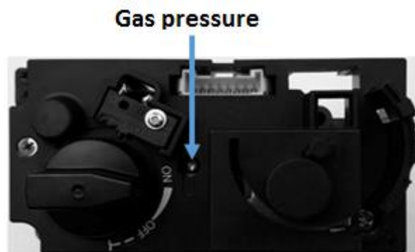
Fig. 21. Method of regulating the outlet pressure
